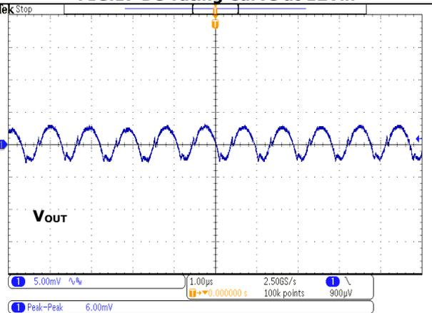
**FIG.19 Output Ripple (12Vin, Iout=3A)**
