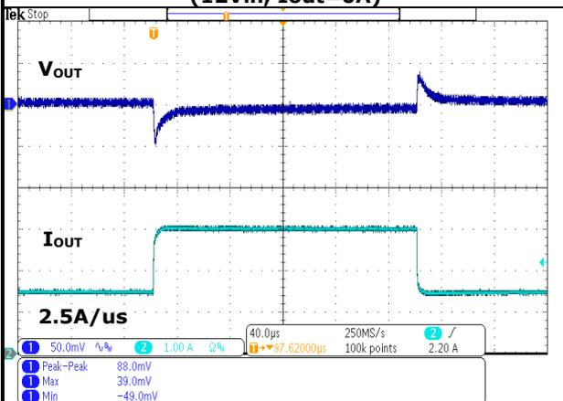
**FIG.20 Transient Response (12Vin, 50% to 100% Load Step)**
