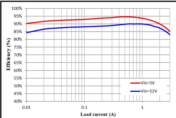
**FIG.16 Efficiency V.S. Load Current**
